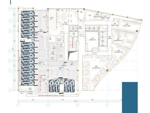
Room dimension for garment storage conveyor from 1,2m width and 1,75m height
